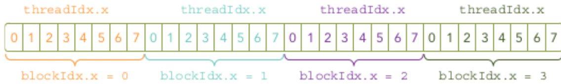
FIGURE 3.6: Thread Alignment for a Typical Kernel Courtesy: Professional CUDA C Programming
