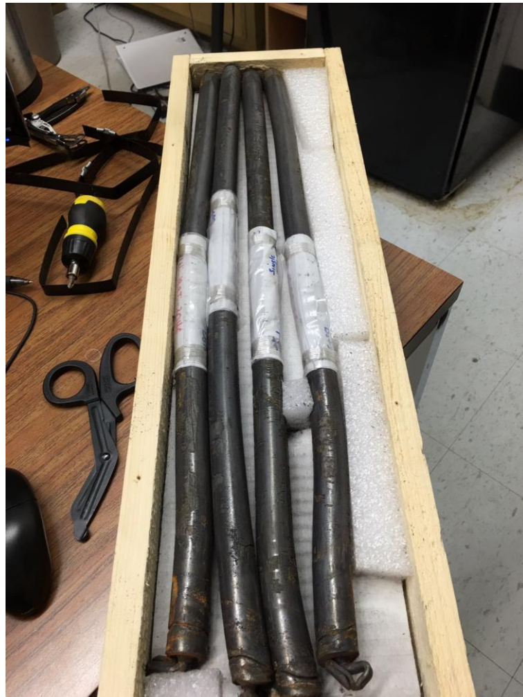
Figure 3.1-1. \text{Ni}_{50.3}\text{Ti}_{29.7}\text{Hf}_{20} alloy after hot extrusion.
