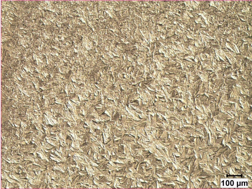
Figure 4.4-3. Optical microscope images of the etched extruded samples after functional fatigue test
