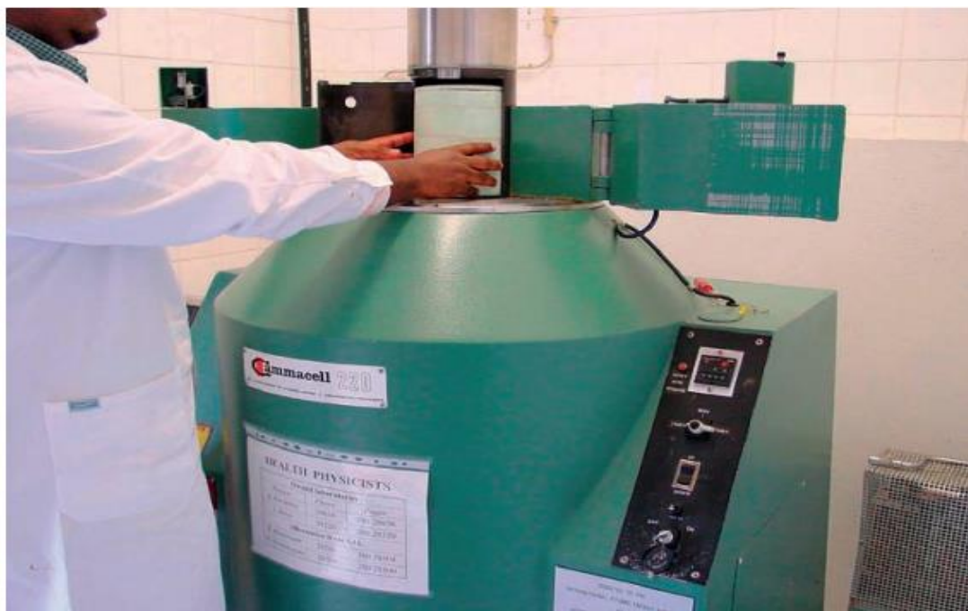
Figure 2.2. Self-contained dry storage gamma irradiator used for research and small dimension materials. (In preparation for irradiation, a sample holder is being placed in the irradiation chamber when it is in the loading position. Depending on the dose rate of the day, the timer on the control panel (bottom right) is set to give the desired dose) (27).
