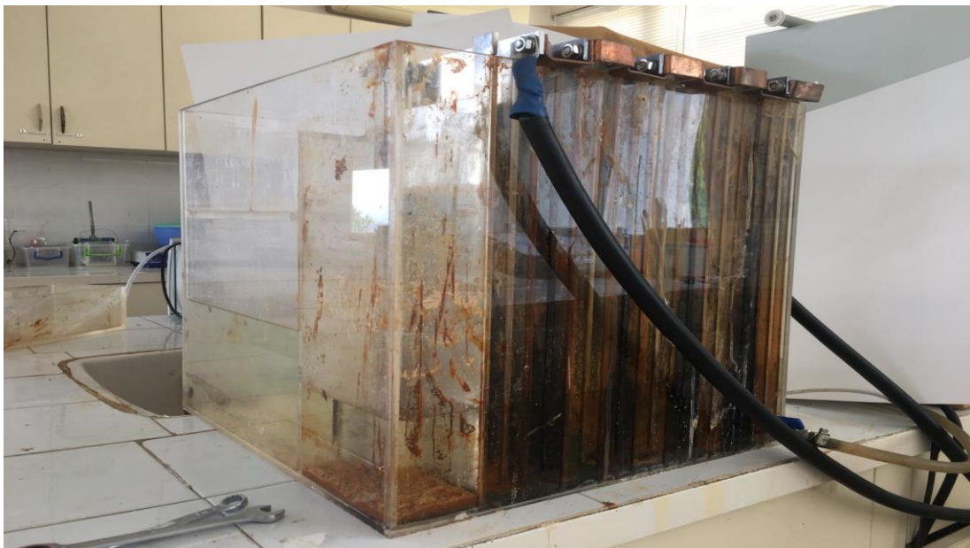
Figure 3.1. Electrode configuration in Electrocoagulation and Electroflocculation reactors.
