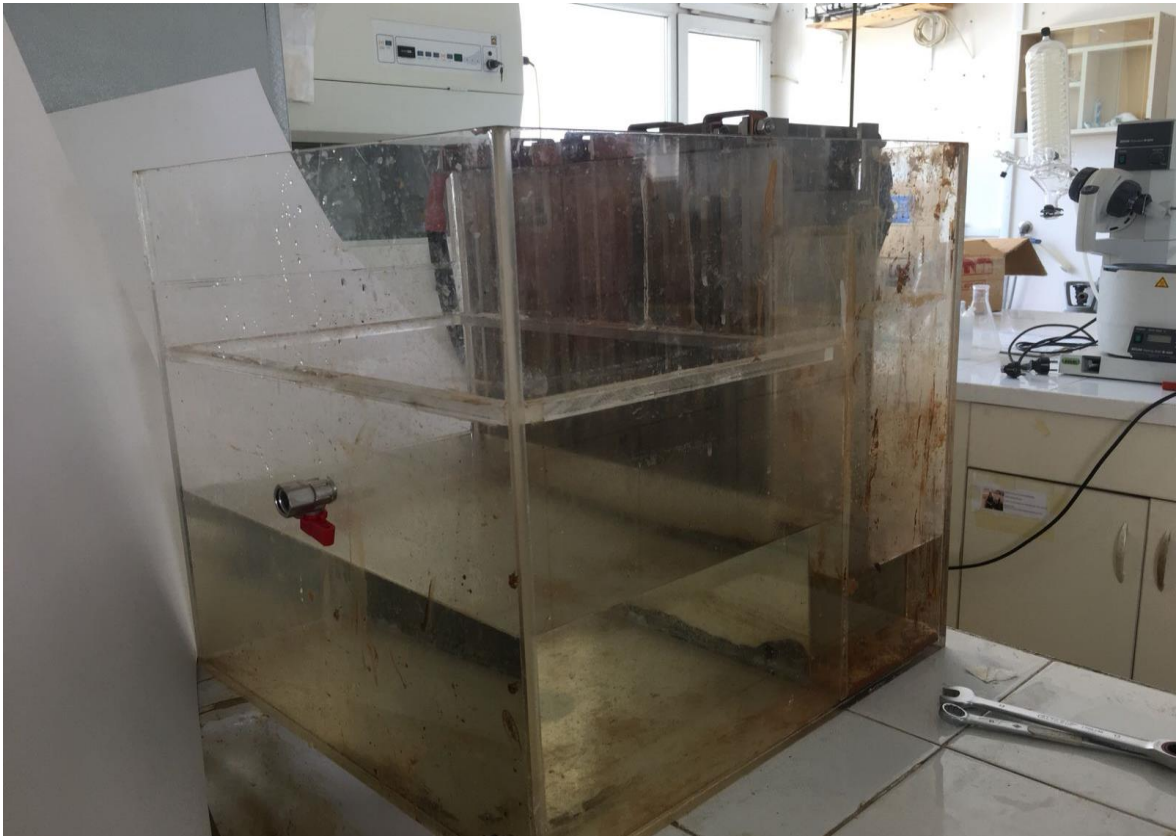
Figure 3.3. Electrocoagulation and Electroflocculation reactors.
