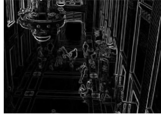
f) \sqrt{\left(\frac{\partial I}{\partial x}\right)^2 + \left(\frac{\partial I}{\partial y}\right)^2}
