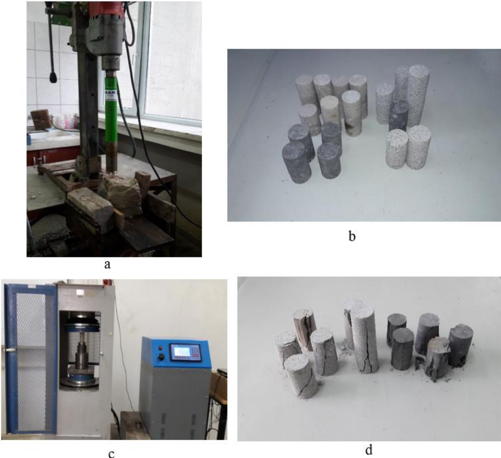
Figure 7.7. Coring machine (a), core samples (b), hydraulic press (c), and the samples after the UCS test (d).
