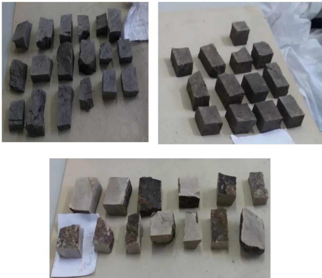
Figure 7.8. Prepared samples for point load test.
