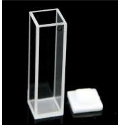
Figure 3.11: Quartz glass cell for particle size measuring
