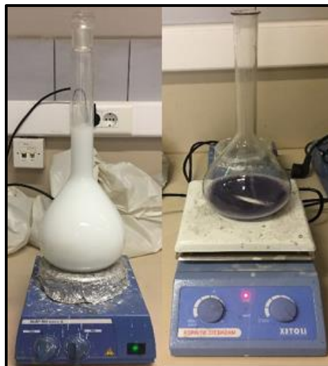
Figure 3.9: Bulk barite sample and bulk fluorite sample prepared for ZP testing
