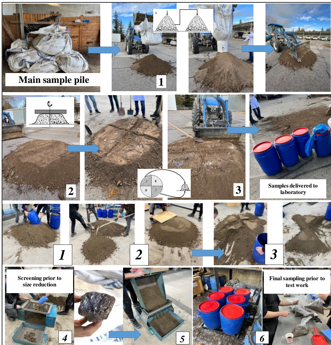
Figure 3.2: Subsequent steps of sampling (1: coning, 2: flattening, 3: quartering, 4: crushing and screening for size reduction, 5: intermediate sampling, 6: packing final sample).
