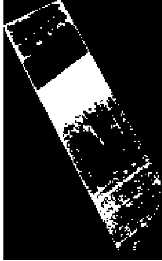
Figure 3.10. Thresholding of the Field #7 image with the value of 51 that was obtained from the histogram
