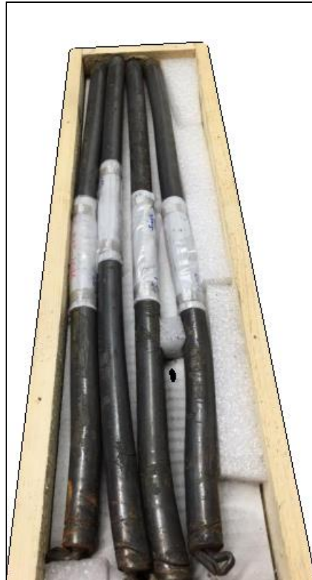
Figure 3.1-1. Hot Extruded Ni 50.1 Ti 19.9 Hf 30 (at%) alloy.
