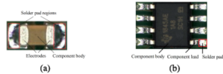
Fig. 1. Surface mount device (SMD) parcellation (a) non-IC component image and its solder pad and component body and (b) IC component image and its body, lead, and solder pad regions.
