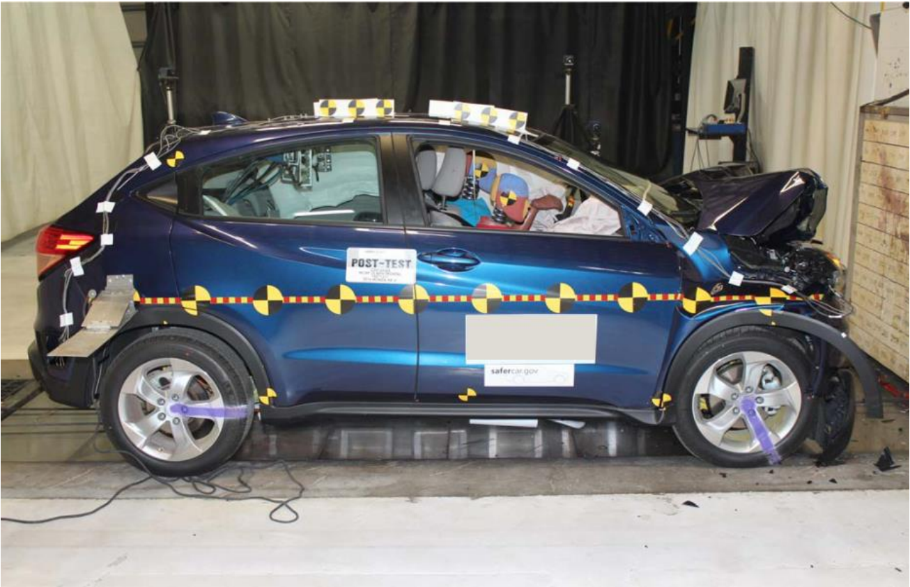
Figure 2: FWRB Frontal Crash Test, Post-Test Right View of Test Vehicle [5]
