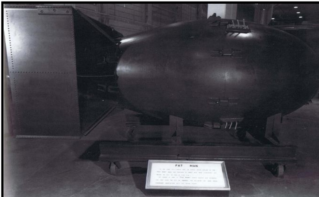
The Fat Man, or Mk-III casing. The Fat Man type was the nuclear free-fall bomb of the United States for four years after Nagasaki. It was used primarily because plutonium was easier to purify than Uranium. Photo by: National Atomic Museum
