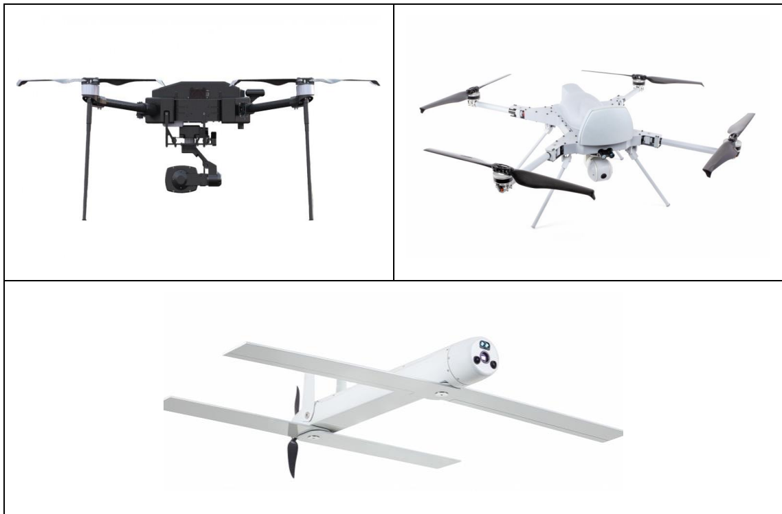
Figure 1-1: Top Left to right, Togan [3] and Kargu [4] rotary wing UAV, bottom Alpagu [5] fixed wing UAV.
