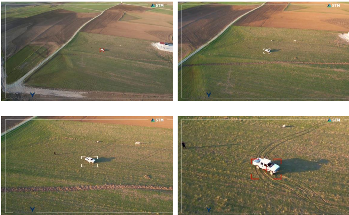
Figure 1-5: Vision system successive target tracking [5]
