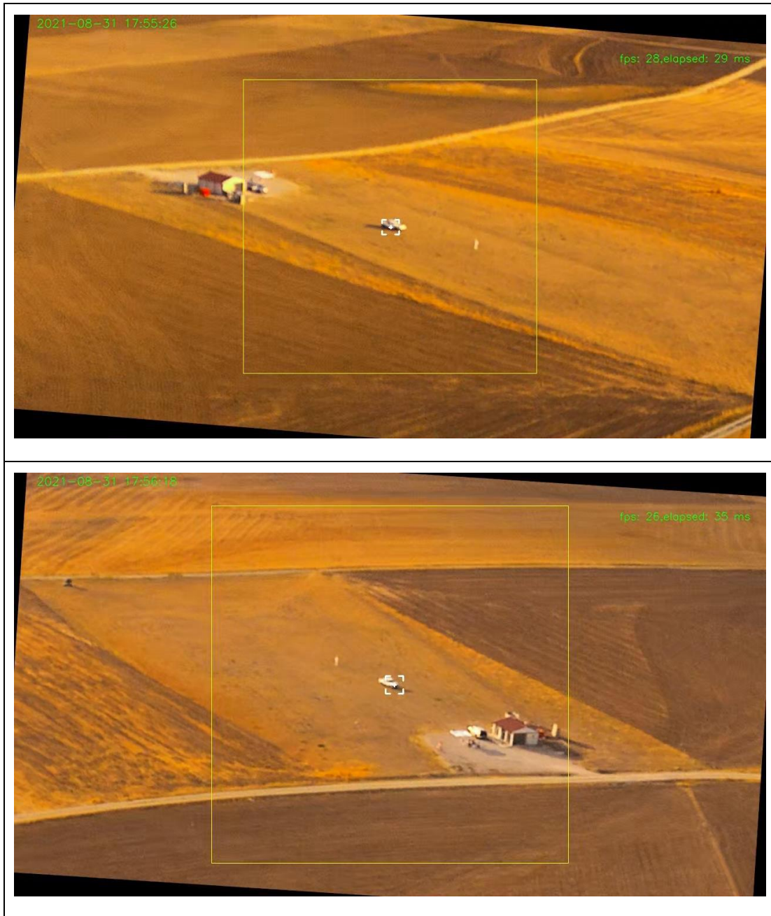
Figure 5-9: Successive target tracking and image-based loitering.
