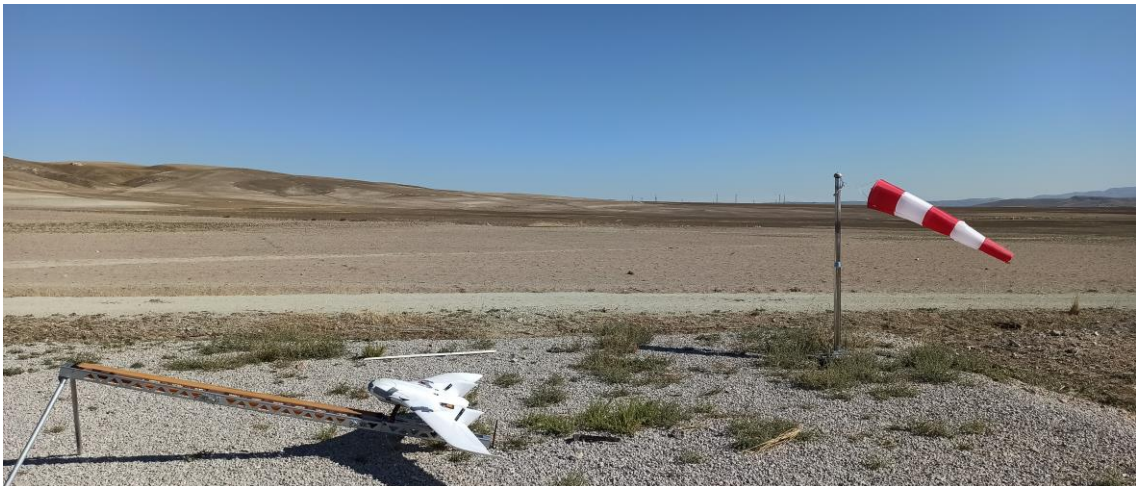
Figure 3-1: Flight test setup, UAV and the launcher
