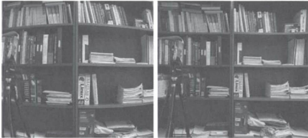
Figure 1-26: Radial distortion effect on image, left with radial distortion [21].
