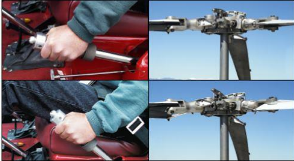
Figure 1.2.2 Collective position and corresponding blade pitch angle [2]
