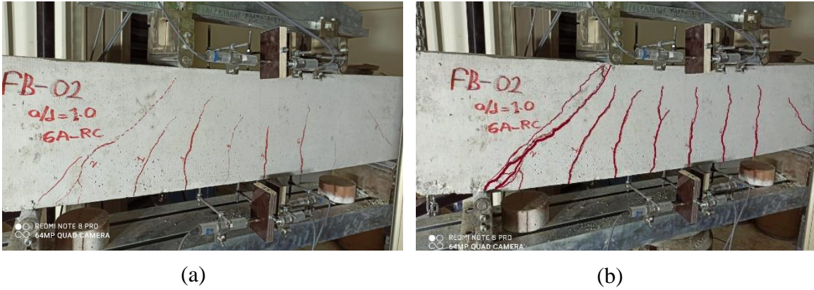
Figure 4.42. CVC – RA – 1.00 beam, (a) first cracks, (b) failure
