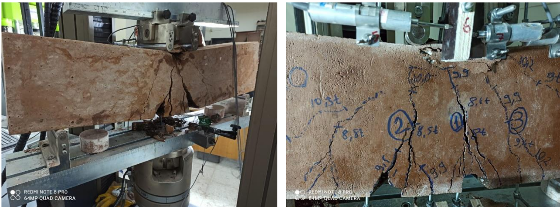
Figure 4.12. GPC – NA – 1.65 beam crushing
