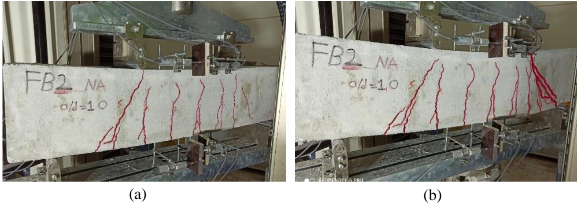
Figure 4.30. CVC – NA – 1.00 beam, (a) first cracks, (b) failure
