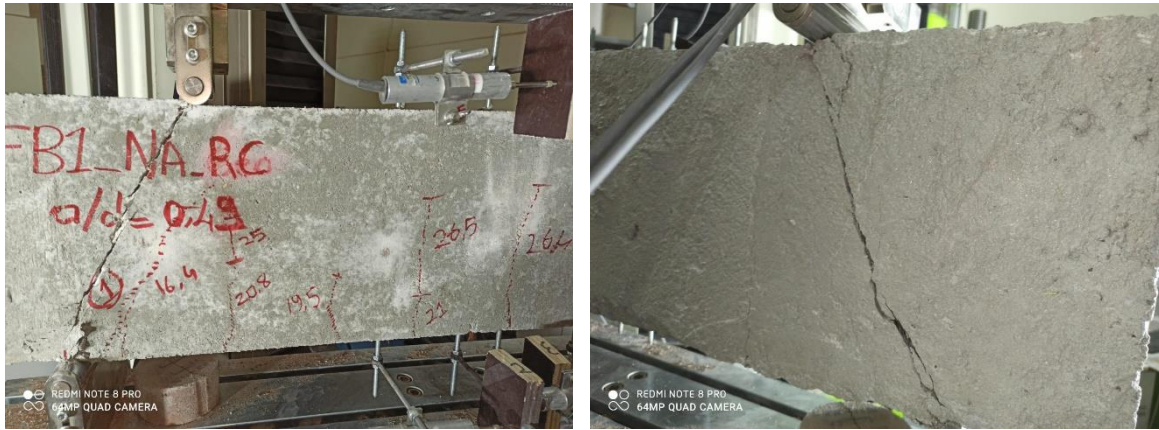
Figure 4.27. CVC – NA – 0.50 failure crack propagation
