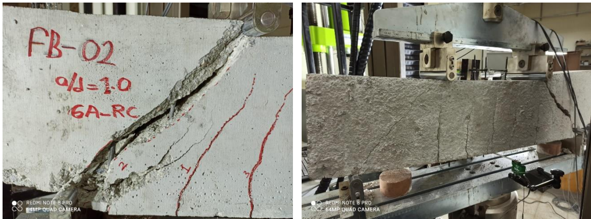
Figure 4.43. CVC – RA – 1.00 shear dominant failure deatiled picture
