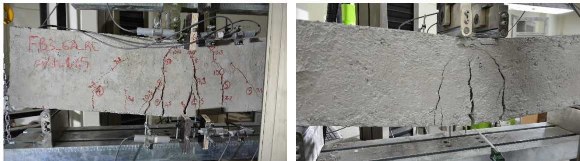
Figure 4.47. CVC – RA – 1.65 flexure dominant failure picture
