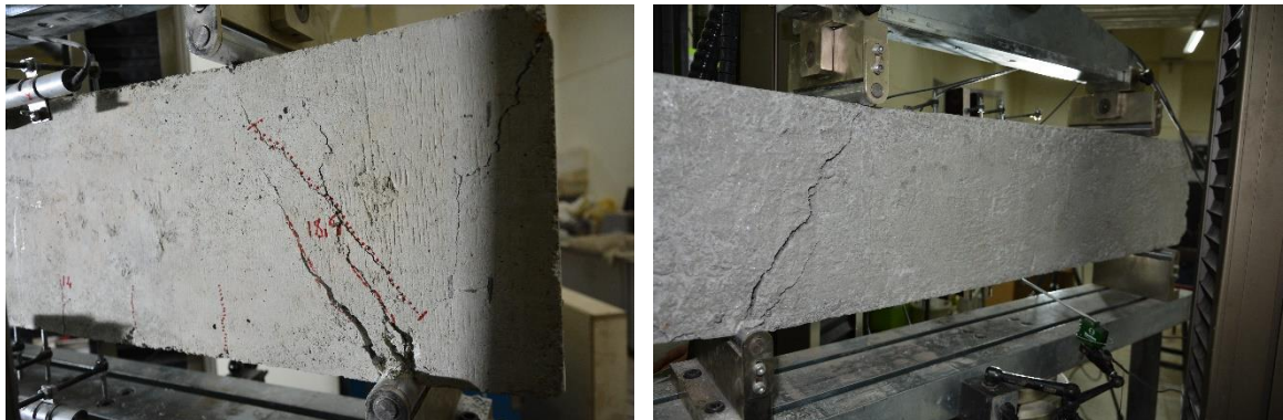
Figure 4.39. CVC – RA – 0.50 shear dominant failure
