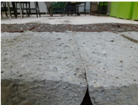
Figure 4.2. Splitting-Tensile Strength Test Setup and Experiment
