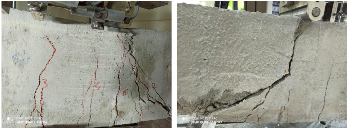
Figure 4.31. CVC – NA – 1.00 shear dominant failure detailed picture
