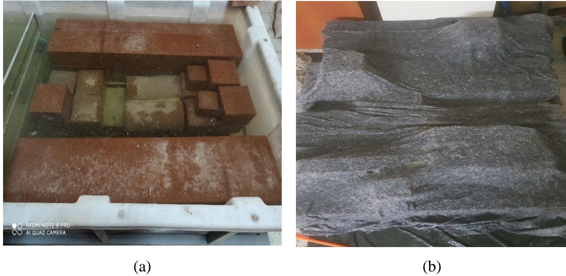
Figure 3.16. Curing of the specimens, (a) geopolymer samples, (b) concrete samples
