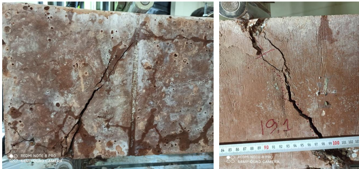
Figure 4.4. GPC – NA – 0.50 shear crack detail
