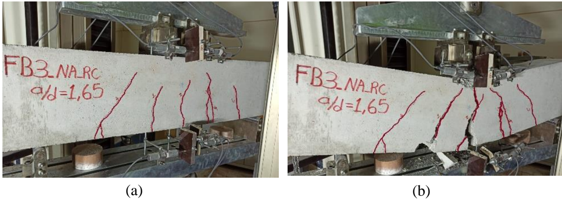
Figure 4.34. CVC – NA – 1.65 beam, (a) first cracks, (b) failure
