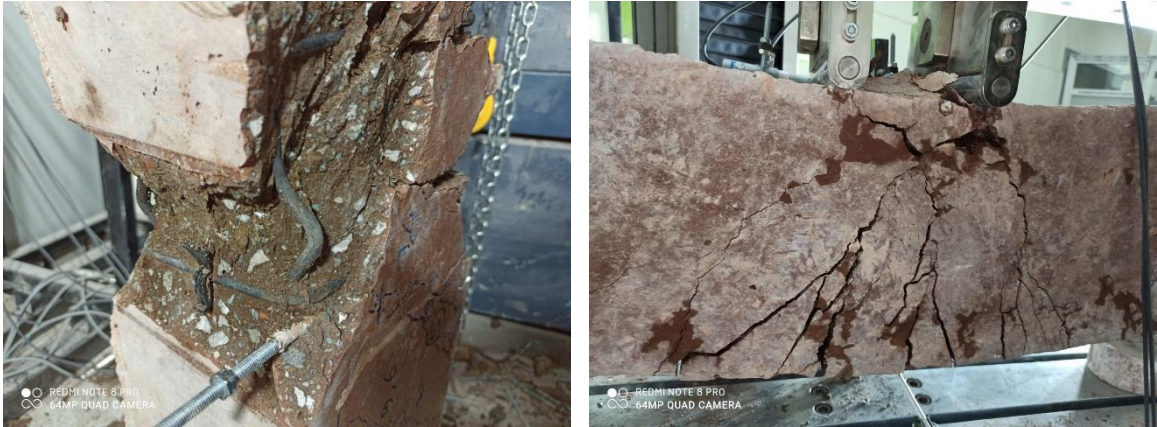
Figure 4.23. GPC – RA – 1.65 buckling of reinforcement bar and crushing of geopolymer
