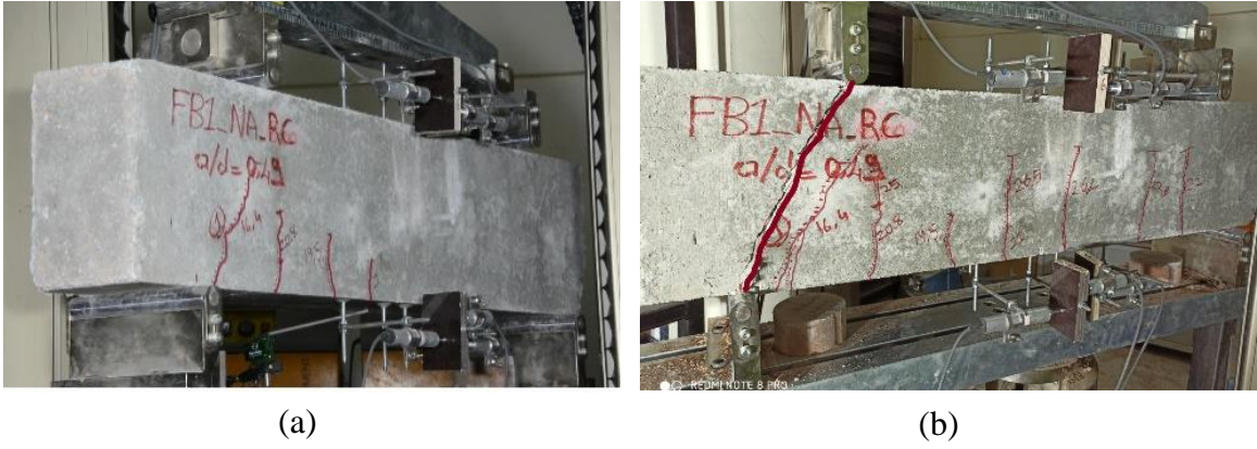
Figure 4.26. CVC – NA – 0.50 beam, (a) first cracks, (b) failure
