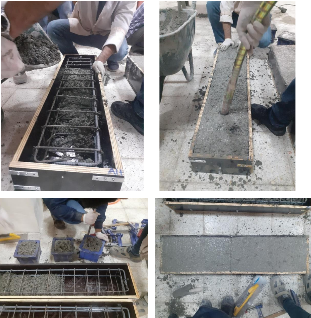
Figure 3.14. Casting and placing procedure of CVC
