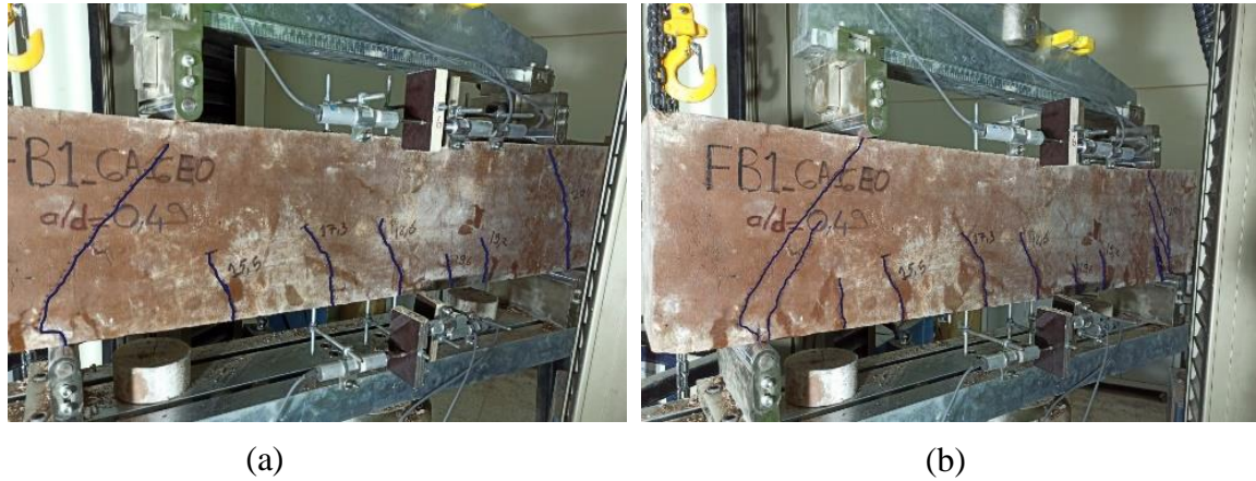
Figure 4.15. GPC – RA – 0.50 beam, (a) first cracks, (b) failure
