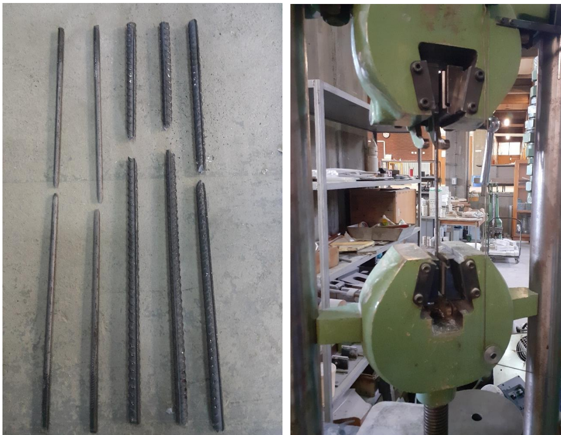
Figure 3.6. Rebar test machine
