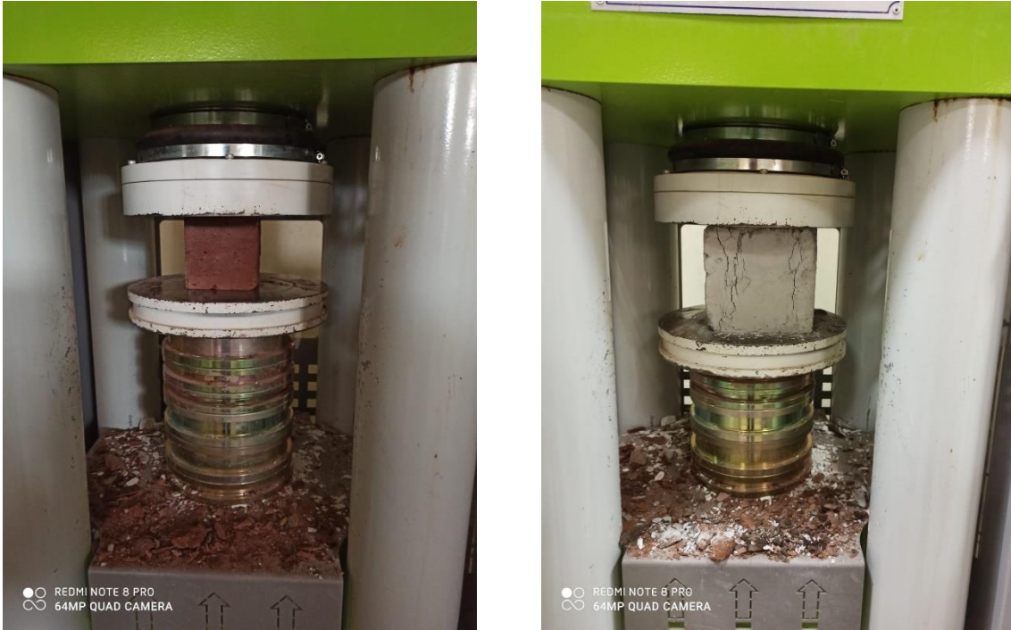
Figure 4.1. Compressive Strength Test Setup and Experiment
