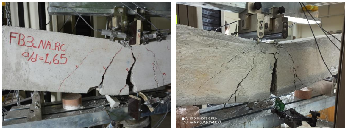
Figure 4.35. CVC – NA – 1.65 flexure dominant failure detailed picture
