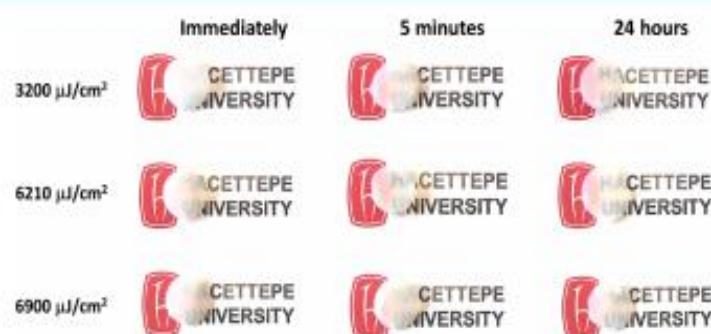
Figure 4. Gross images indicative of the effects of different exposure densities and impregnation times on transparency. Materials were exposed to 3200, 6210, and 6900 \mu\text{J}/\text{cm}^2 UV light (365 nm) for 1.5 min with 10 s intervals up to 6 times: immediately cross-linked constructs after impregnation on GelMA solution (Immediately), cross-linked constructs after 5 min (5 minutes), and after 24 h of impregnation (24 hours).
