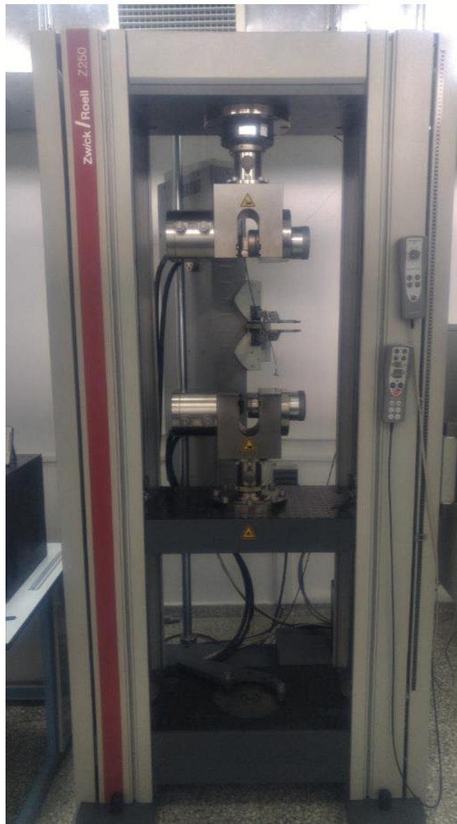
Figure 3.31. Testing Machine Zwick Roell Z250
