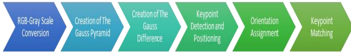
Figure 4.3. SIFT algorithm flowchart
