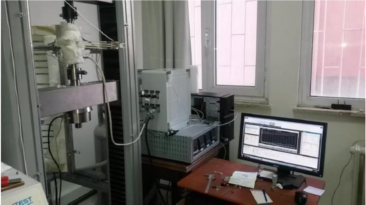
Figure 3.6-1. Load-biased heating-cooling test equipment.
