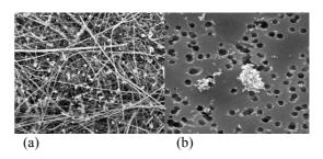
**Fig. 1.** SEM images of the sample loaded glass fiber filters of Kayaş-1 (100 fold magnification) (a) and sample loaded poly carbonate fine filter Beytepe 1 (3000 fold magnification, particle size  $< 2.5 \ \mu\text{m}$ ) (b).
