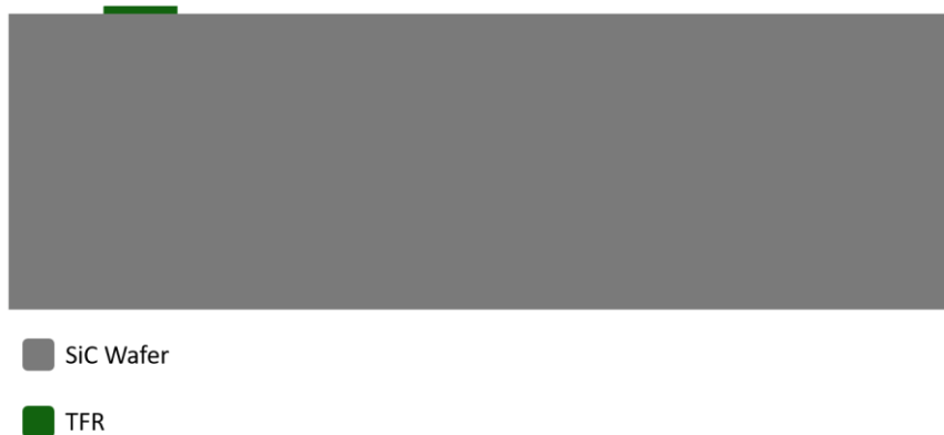
Figure 6.2 Cross-section of wafer after TFR coating
