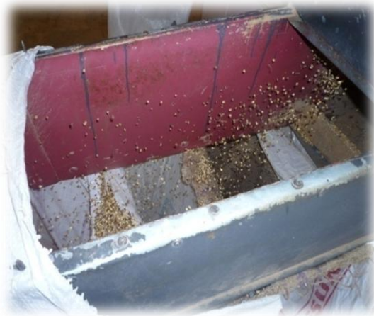
Figure 3.4. The separation of kernels from cracked dried fruits by air pumping
