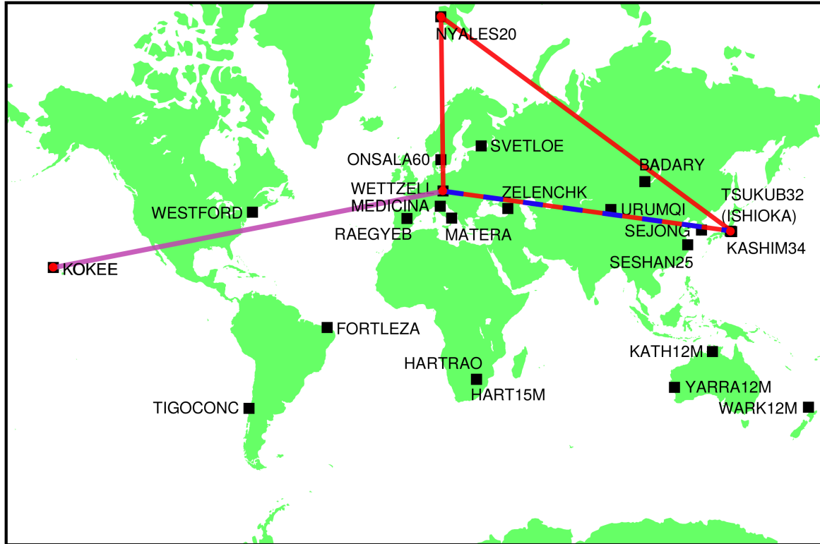
Figure 7.1: VLBI stations participating in IVS-R1 and -R4 sessions (black squares) as well as Intensives (red dots). INT1, INT2, and INT3 baseline vectors are given with purple, blue (dashed) and red lines, respectively.
