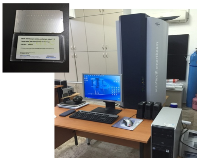
Figure 3.4. The MALDI-TOF MS system used in this study by Bruker (Germany). The target plate with 384 spots used is on the top left.
