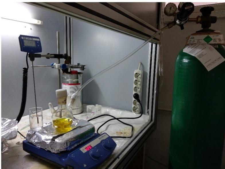
Figure 3.4. Apparatus for the synthesis of SPIONs
