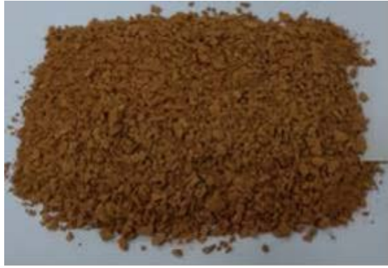
Crushed hollow brick
