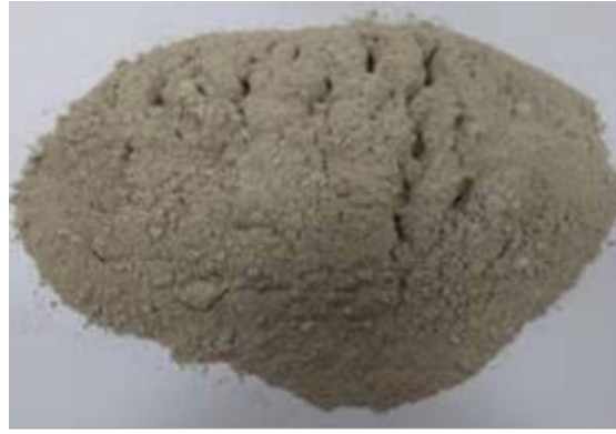
Ground concrete waste
