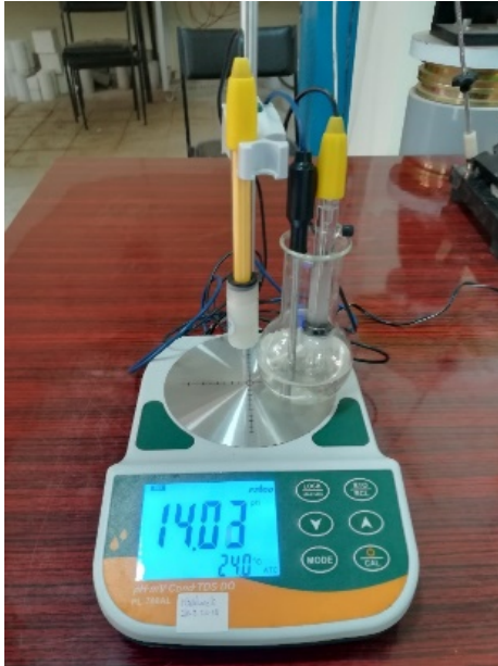
Figure 3.12 Measuring pH values of various alkali activator solutions
