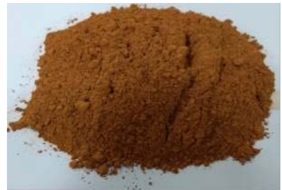
Ground roof tile
