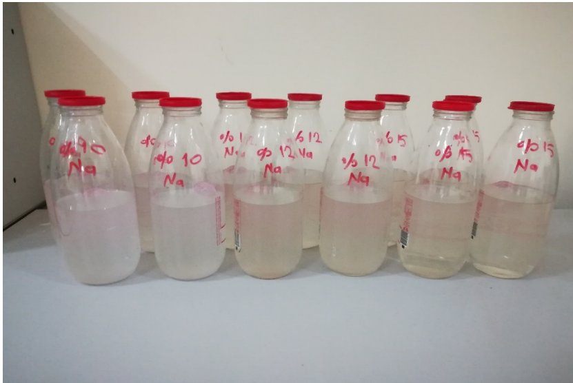
Figure 4.1 Process of cooling the solutions of various alkaline activators in glass bottles
