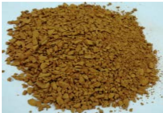
Crushed roof tile
