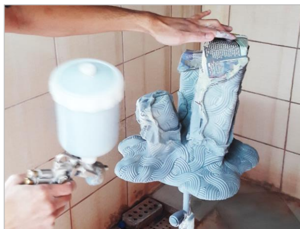
Figure 76: Glazing process using spray technique (Yahya Daud Ismail, 2018).
