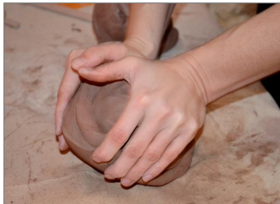
Figure 67: Wedging process to remove air pockets in clay. Photo by Kate (2011).
