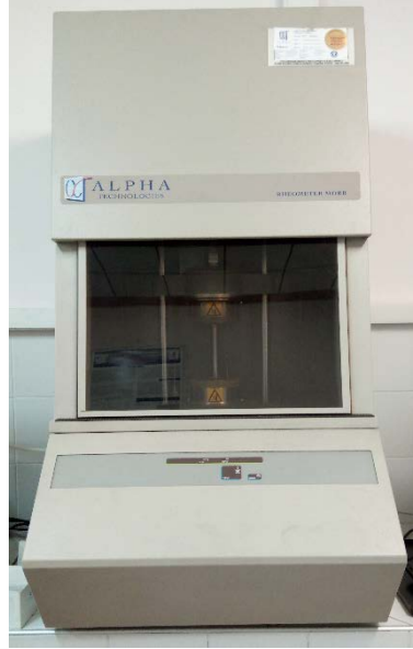
Şekil 3.2. Alpha Technologies MDR 2000B
