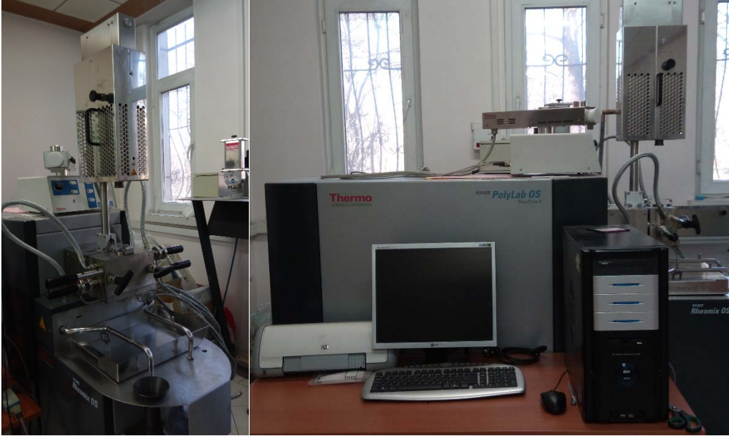
Őekil 3.1. Thermo HAAKE Rheomix Tork Reometre
