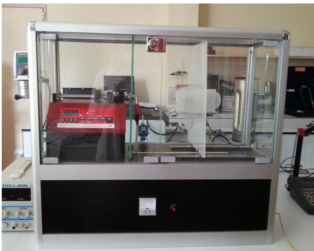
Figure 2.1. Electrospinning setup in our laboratory
