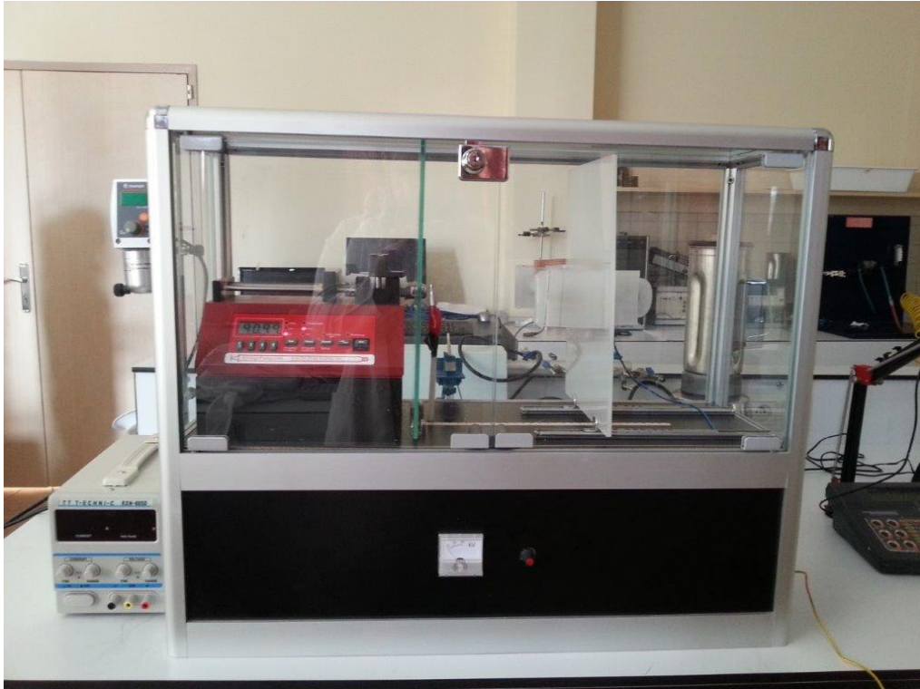
Figure 3.1. Typical electrospinning set up in our laboratory
