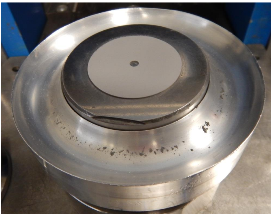
Figure 21. Compacted pyrotechnic mixture (heat pellet)
