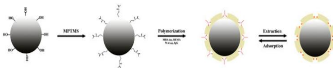
Figure 2.10. Steps of of Con A polymerization process by core-shell imprinted silica particles [38].
