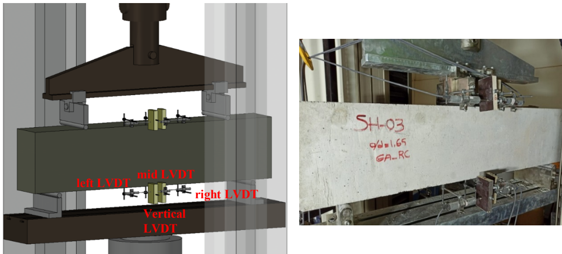
Fig. 2.2. Schematic view of the four-point bending test and the instrumentations [125]
