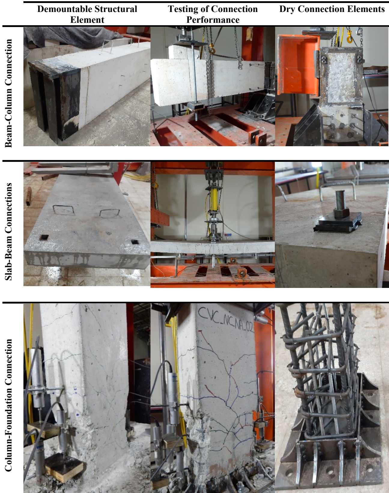
Fig. 1.4. Demountable structural elements and connections
