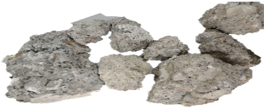
Figure 3. 2. Concrete rubble for the purpose of crushing
