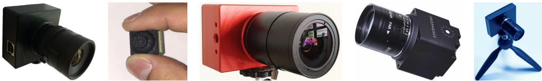
Figure 2.1 Pictures of example event cameras. From left to right: DVS128, miniDVS, and DAVIS346 by iniVation, EVK4 from PROPHESEE, and CeleX-V from CelePixel Technology.
