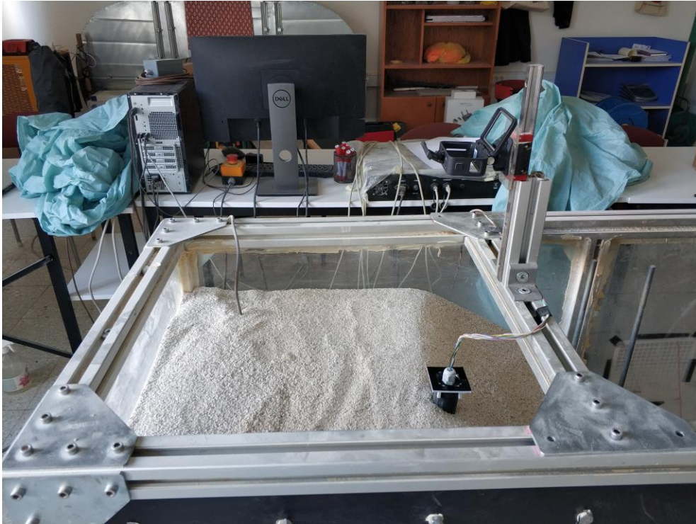
Figure 24. Camera stand mounted on the landslide container
