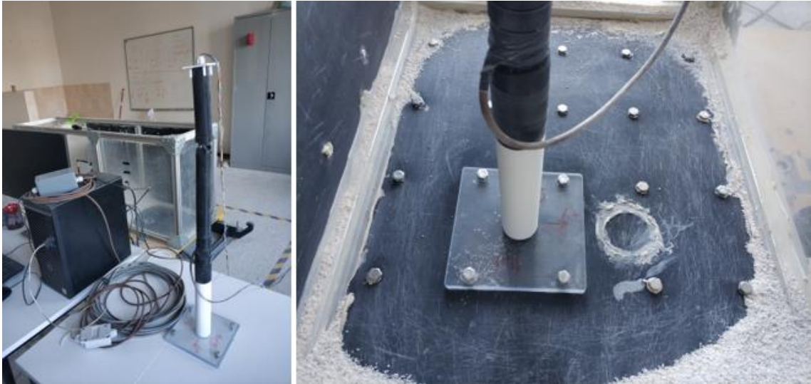
Figure 29. Tilt sensor cable connections and mounting of the tilting pipe on the shaking table
