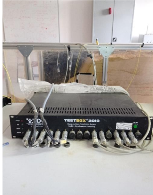
Figure 22. Data logger that is connected to shake table
