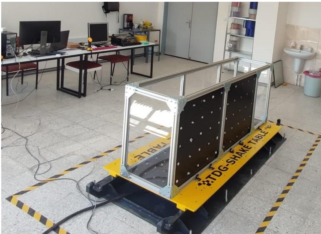
Figure 20. View of landslide container and shaking table after installation
