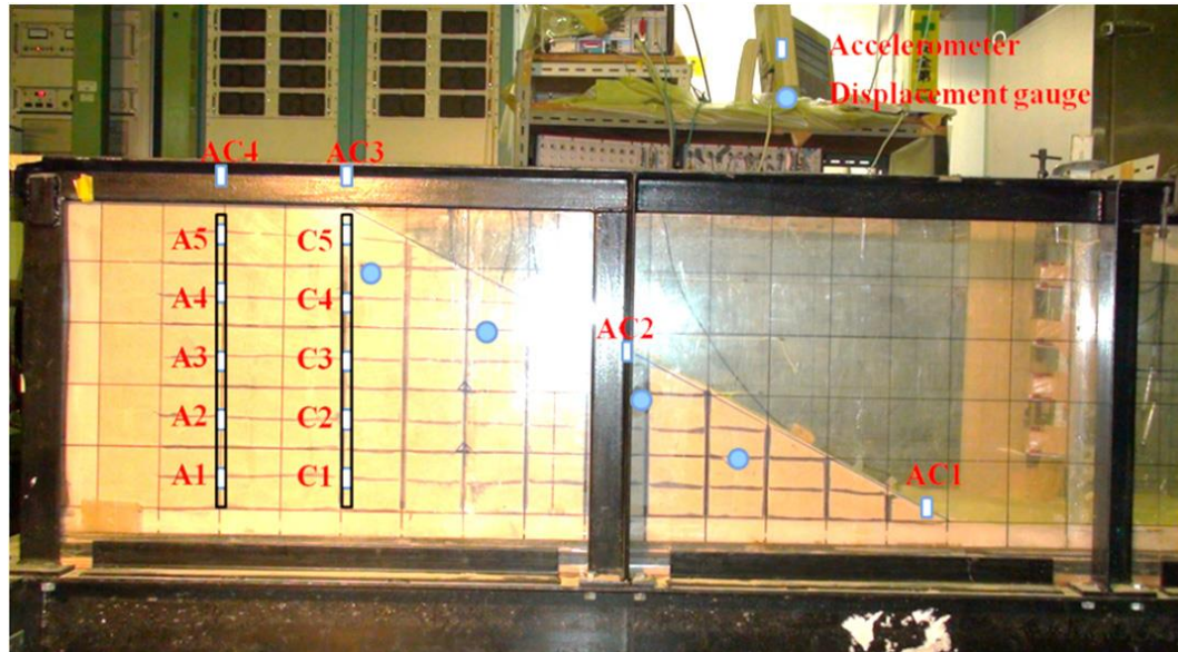
Figure 5. Slope model with accelerometers and displacement gauges (Zhao et al., 2015)
