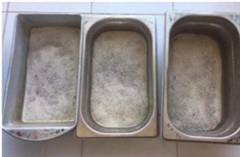
Figure 4.11. Obtained \text{CaCO}_3 in f-RCA sand mixes after the microbial treatment with 0.3 \text{ g CDW.L}^{-1}
