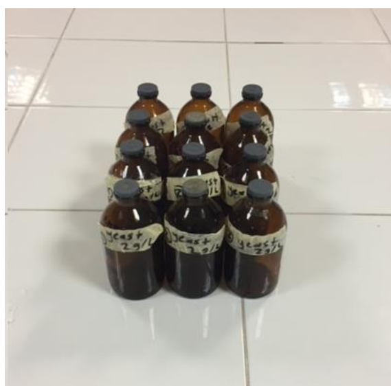
Figure 3.7. Batch tests for investigating the effect of yeast extract on microbial activity
