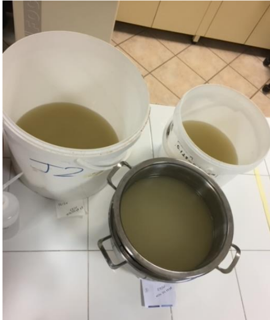
Figure 3.6. Experimental setup for treatment of f-RCA sand mix
