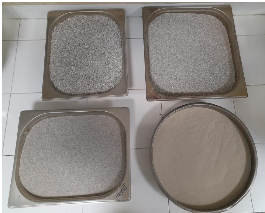
Figure 3.3. The four different size groups of f-RCA used in the sand mix
