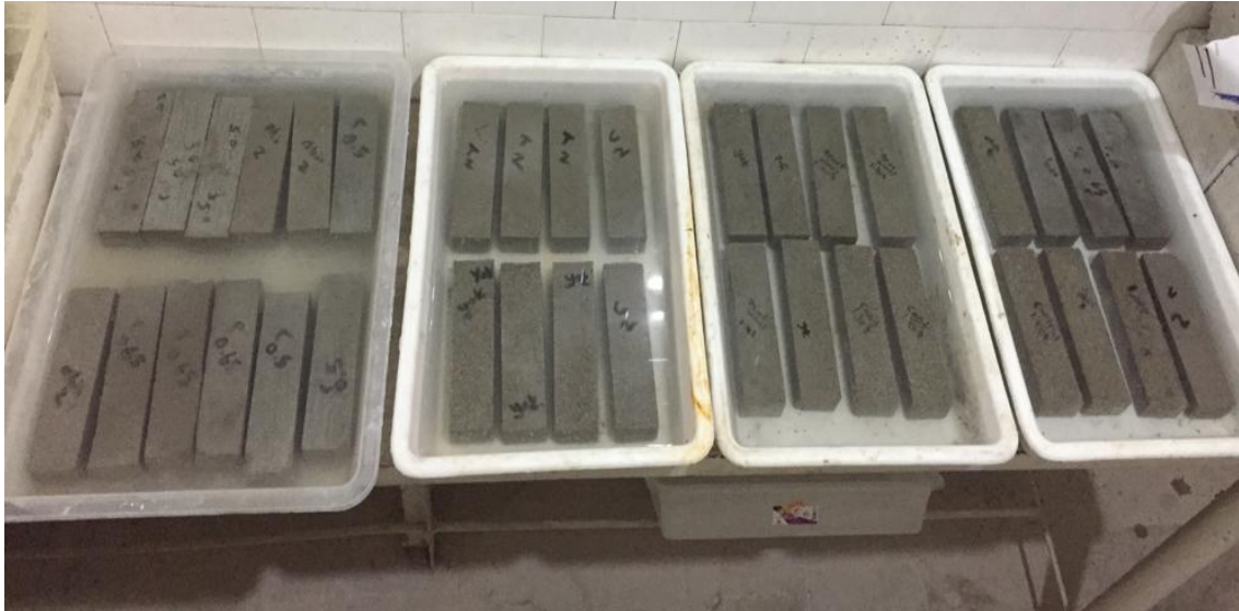
Figure 3.9. Water cured beam mortar specimens
