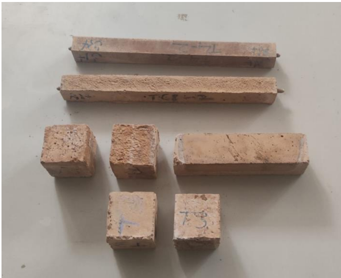
Figure 3.9. Digital images of samples cured under ambient conditions.
