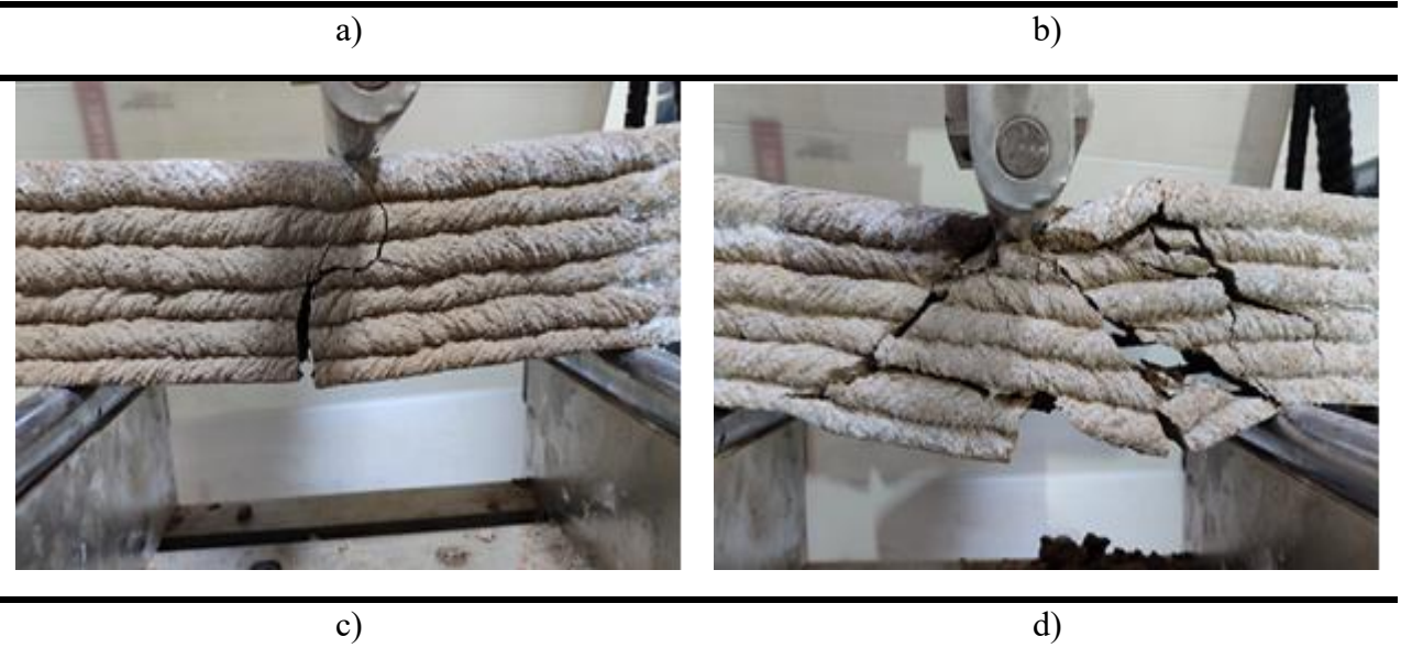
Figure 4.33. Typical failure patterns of bended specimens a) BS specimen, b) BS-FR specimen, c) BS-SSR specimen, d) BS-MSR specimen.
