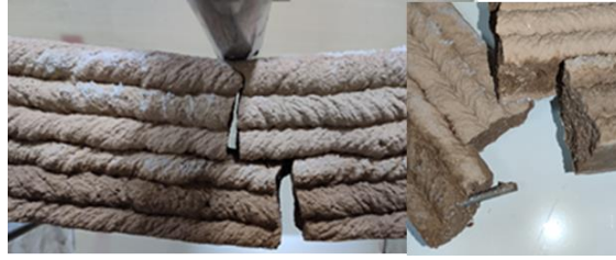
Figure 4.37. Typical failure patterns of bended specimens a) FCA specimen, b) PCA specimen, c) PCA-W specimen, d) PCA-C specimen, e) PCA-S specimen.
