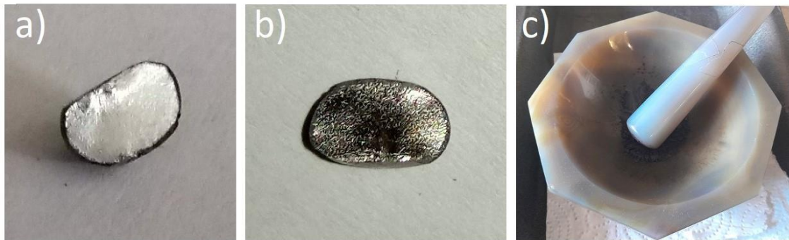
Figure 5.1. a-b) Crushed LaFeSi samples, c) powdering step.
