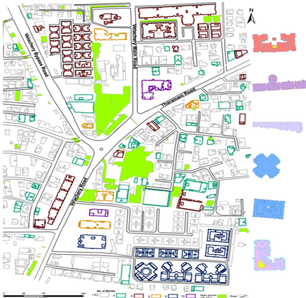
Figure 2.1. Detection of the irregularity in the plan and the floor height of the building from satellite images. (Rajarithnam and Santhakumar, 2015)
