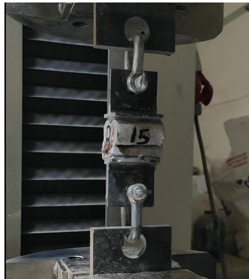
Figure 3.13. Schematic depiction of direct tensile test (a) and representative images from experiments (b).
