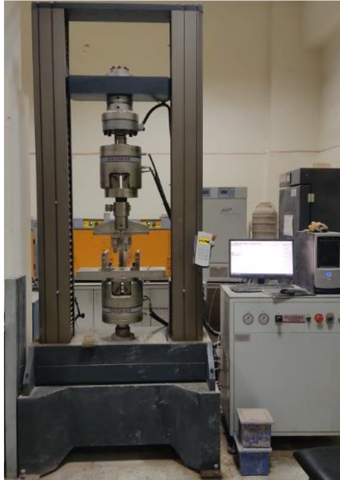
Figure 3.11. Displacement controlled test machine.
