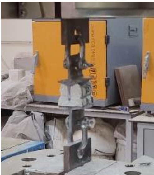
Figure 3.13. Schematic depiction of direct tensile test (a) and representative images from experiments (b).
