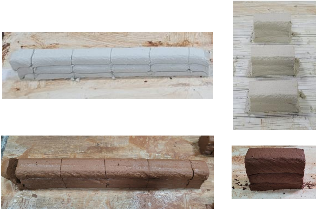
Figure 3.8. The freshly printed mixtures and the subsequently extracted specimens.
