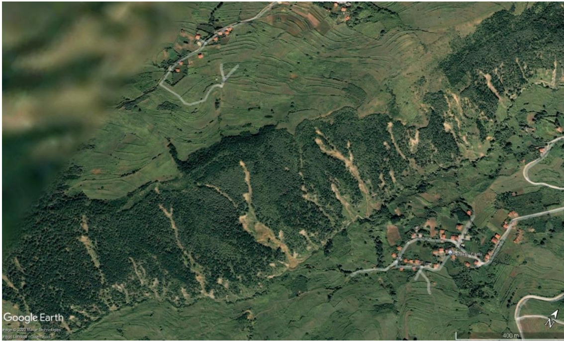
Figure 4.1. Some typical triggered shallow landslides view in the study area after May 1998 rainfall from Google Earth image.
