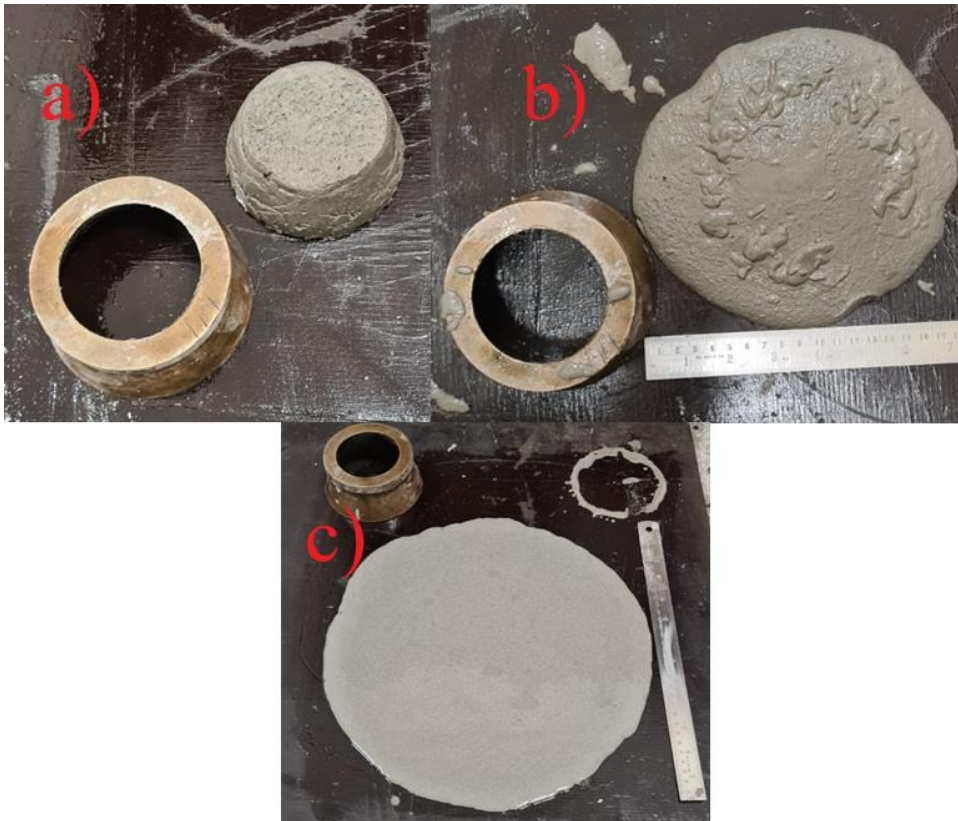
Figure 33 Mini slump tests for the composites a) T-0.3-7-C0.5 b) T-0.3-7-C1.0 c) T-0.3-7-C2
