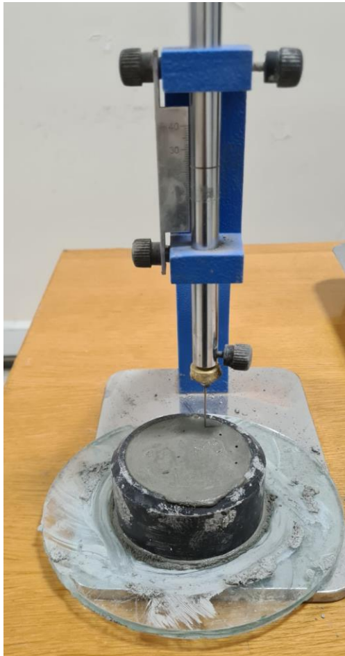
Figure 22 Setting time test via Vicat needle.
