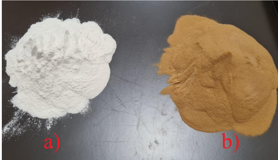
Figure 13 Digital image of the superplasticizers used in the study a) polycarboxylate-based CEMESTE P 97-H b) naphthalene-based SP
