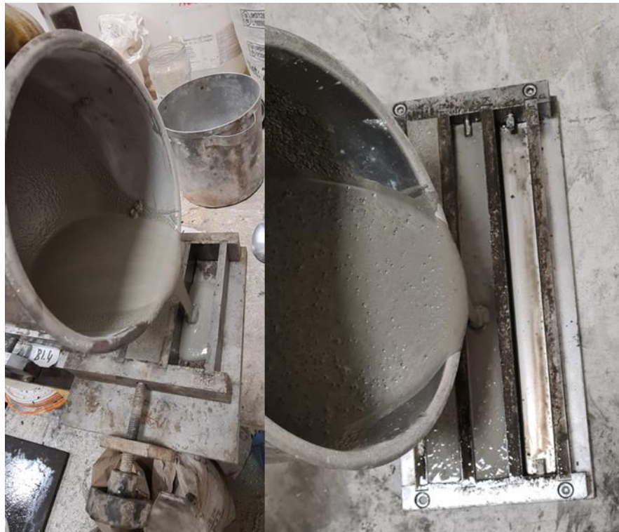
Figure 20 Pouring self-compacting mixtures in formworks.
