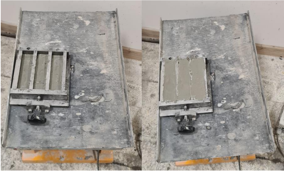
Figure 19 Samples placed to formworks by using the vibrating table.
