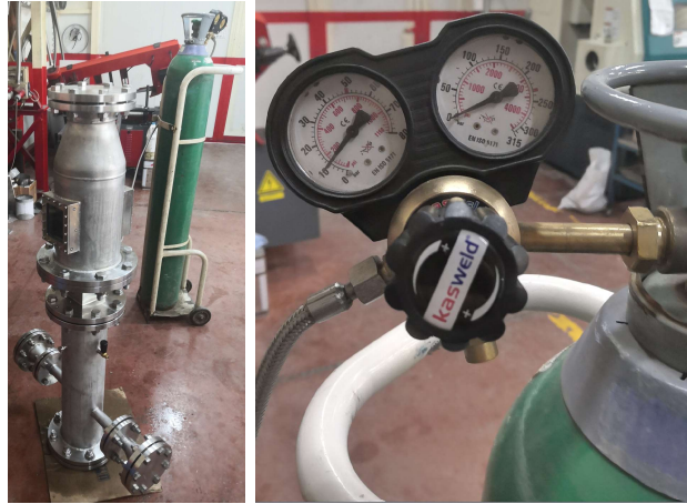
Figure 2.27. View of produced test setup and testing process (endurance and leakage).
