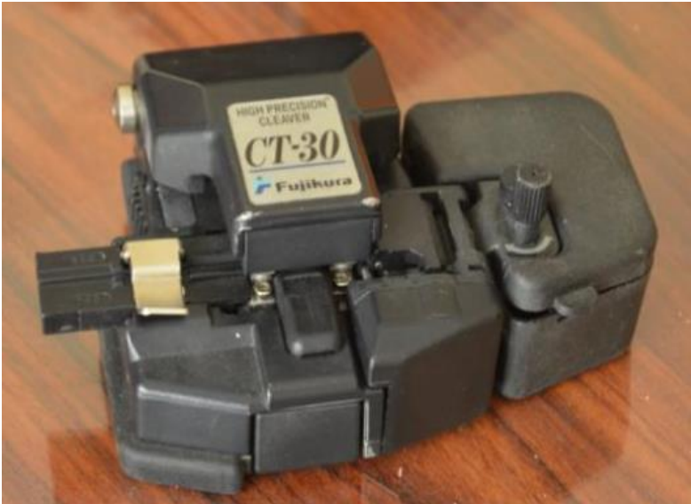
Figure 46. A view of the cleaver used to cut the fiber cables properly
