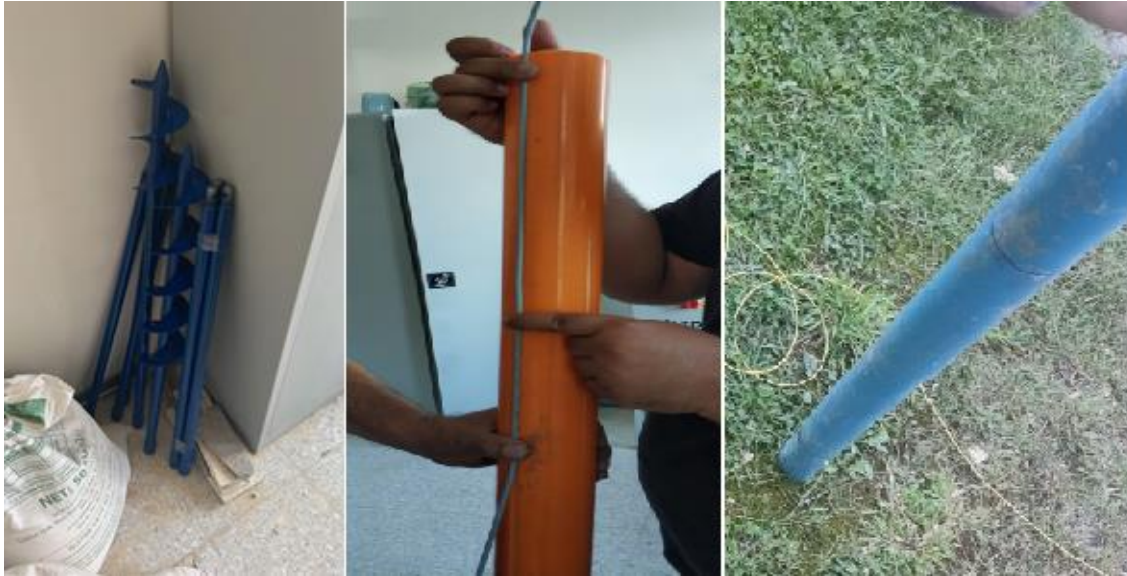
Figure 15. Hand auger and inclinometer pipes
