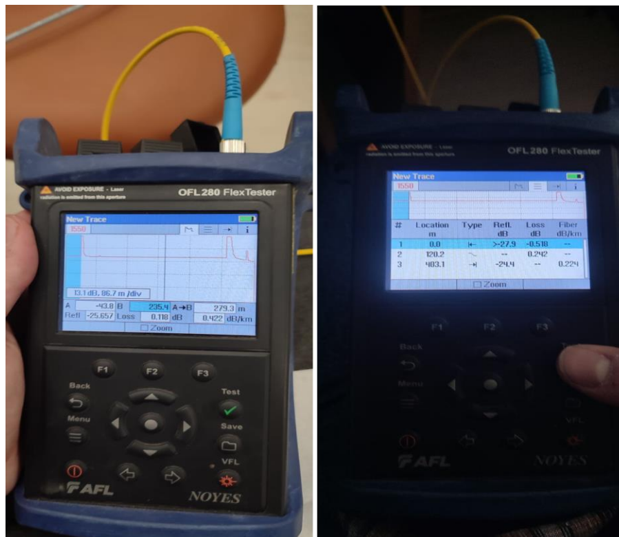
Figure 44. The energy loss check of fiber optic cable by OTDR
