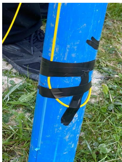
Figure 17. The view of the small channels on the inclinometer pipe
