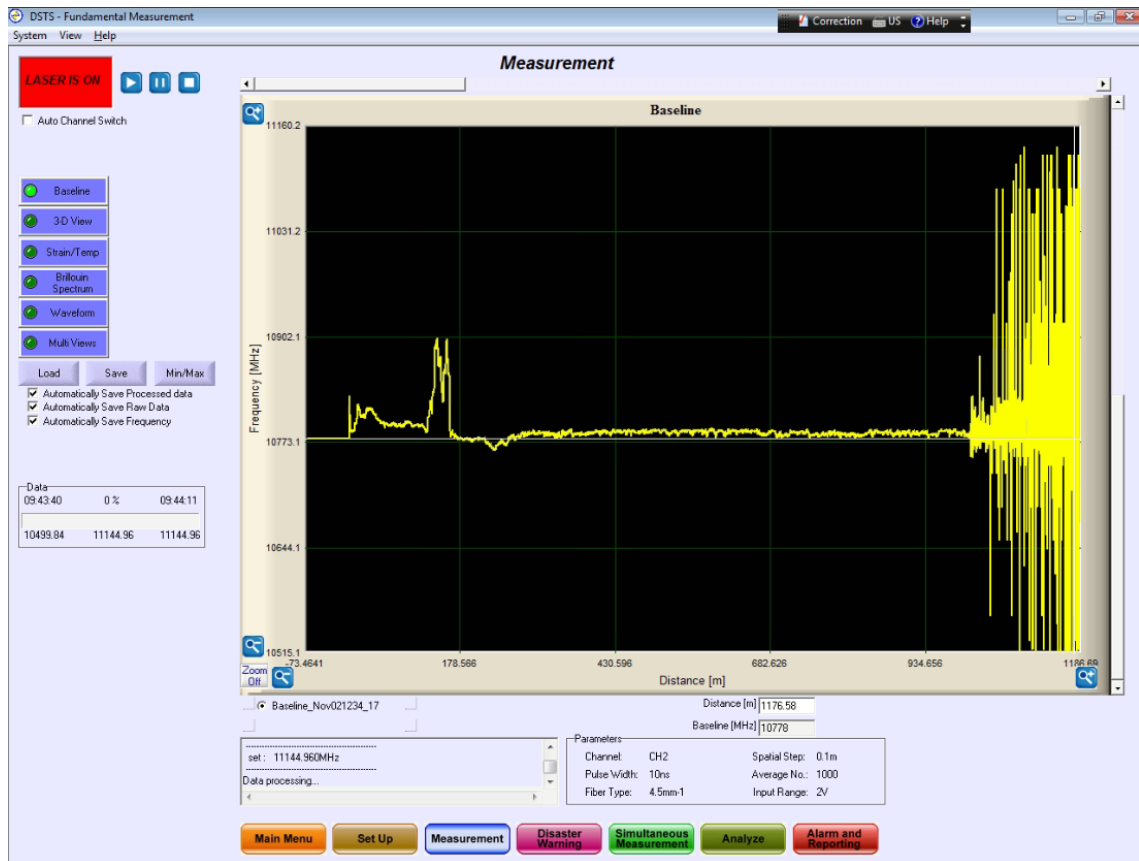
Figure 34. Fiber optic system interface showing baseline measurement of fiber optical cable
