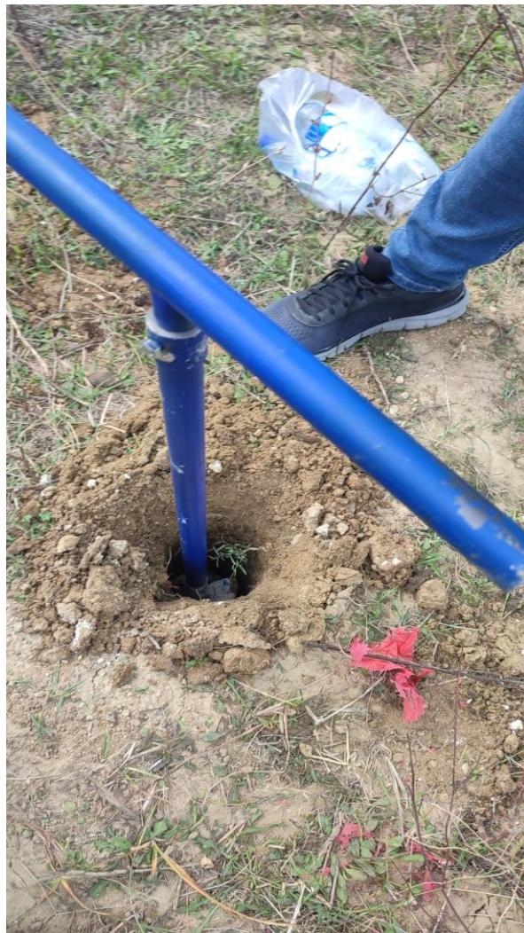
Figure 35. Boring applications with the hand auger method
