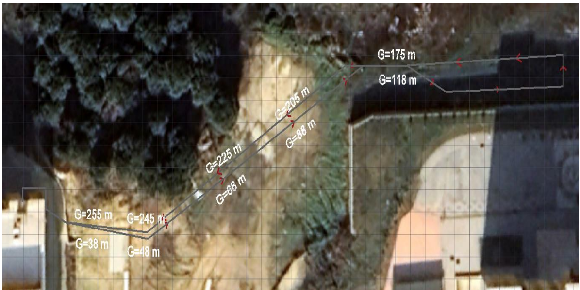
Figure 48. Site installation configuration of 4.5-mm fiber optical cable (gray cable)
