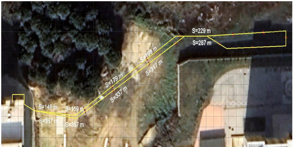
Figure 47. Site installation configuration of 3-mm fiber optical cable (yellow cable)
