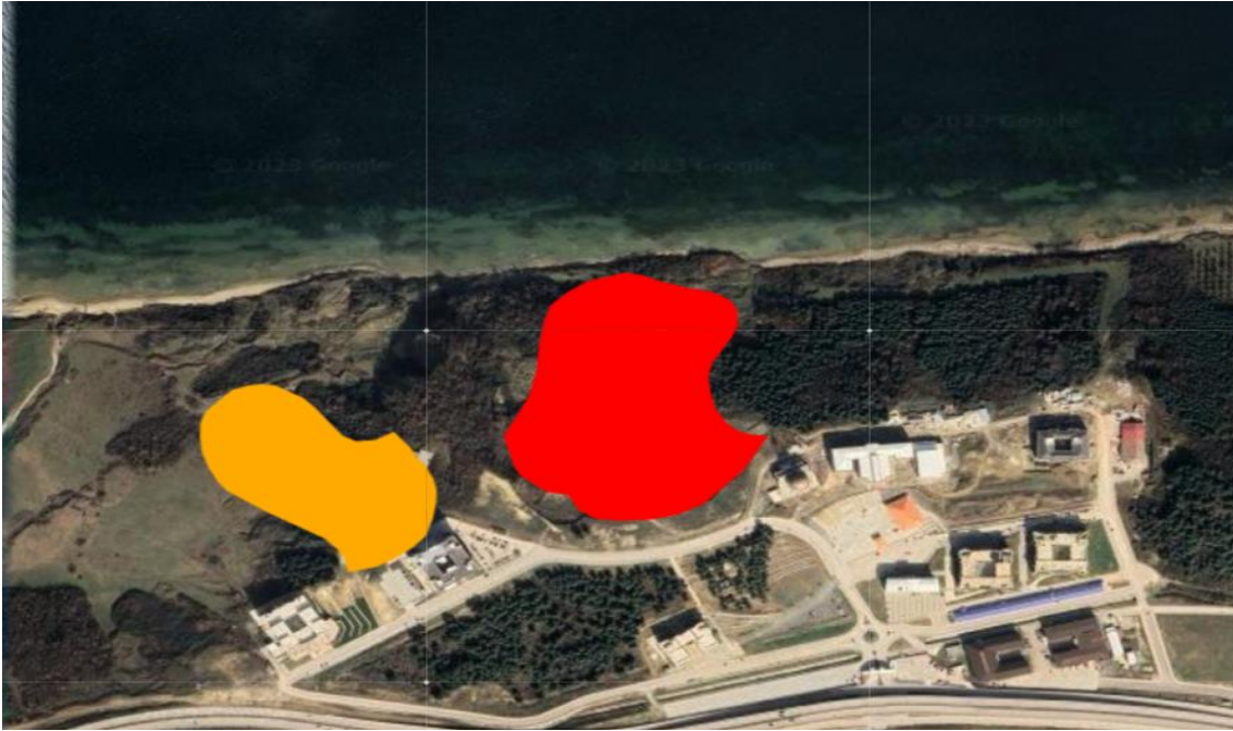
Figure 24. Landslide Map of the study area: Red represents an active landslide, and orange represents the susceptible slope for a landslide. (Geosciences Map, General Directorate of Mineral Research and Exploration, MTA, 2021)
