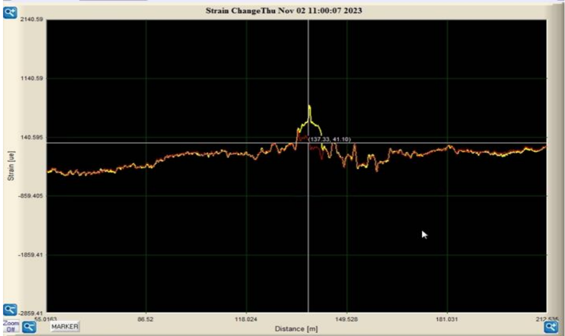
Figure 57. Strain variation with 4.5-mm fiber cable during the tensile operation to BH 6
