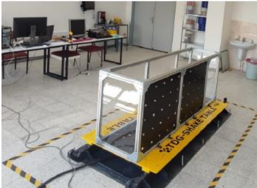
Figure 13. Landslide Container and Shake Table
