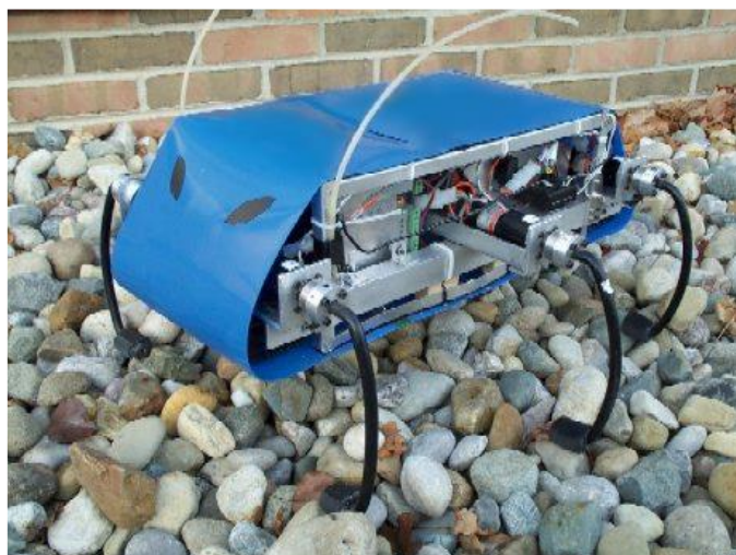
Figure 2.1. First Experimental Rhex Robot [2]
