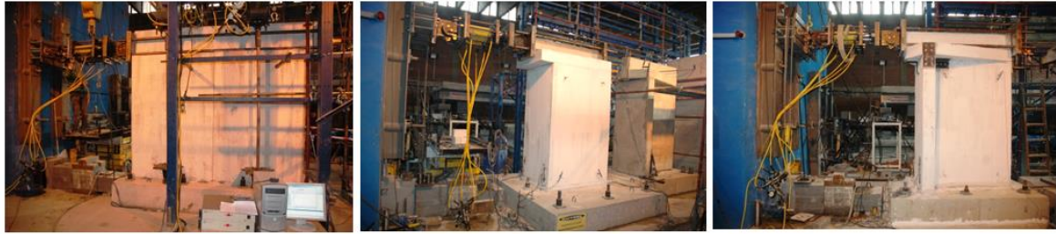
Figure 2.4. Photos from the experimental setup of the shear wall specimens in Aldemir et al.
