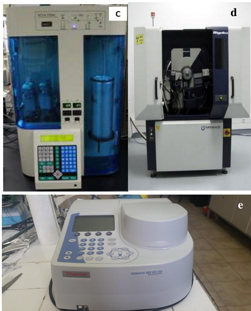
Figure 3.1. The equipment used for the characterization of bare chitosan microgel beads, bare TiO 2 spheres, gold nanoparticles and heterogeneous catalysts a) QUANTA 400F Field Emission SEM-EDAX b) CTEM, FEI Tecnai G2 Spirit BioTwin c) Surface Area and Pore Size Analyzer, Quantachrome Nova 2200 d) XRD, Rigaku Ultima IV e) UV-Vis Spectrophotometer, GENESYS 10S, Thermo Scientific
