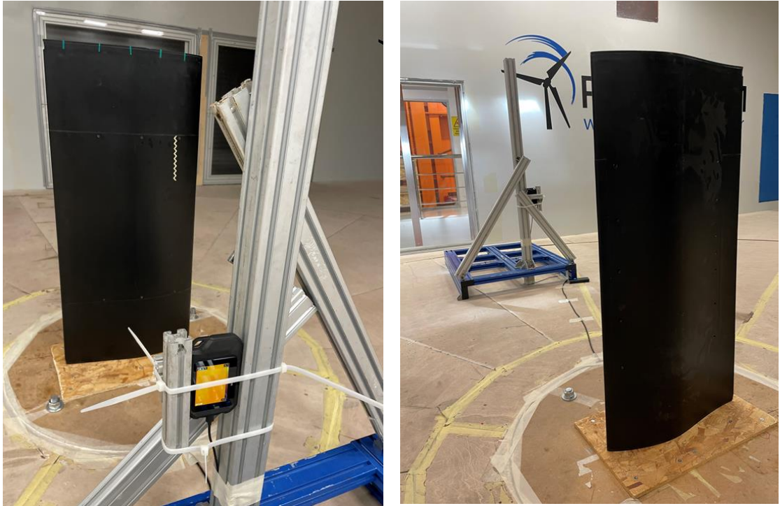
Figure 2.7. Positions of the airfoil and IR camera in the TS2
