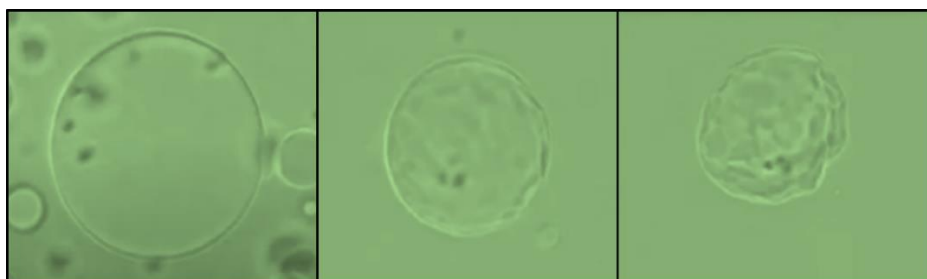
Figure 4.15. Shrinkage behavior of droplet formed by ZrCl_4 +DMF solution in silicone oil.
