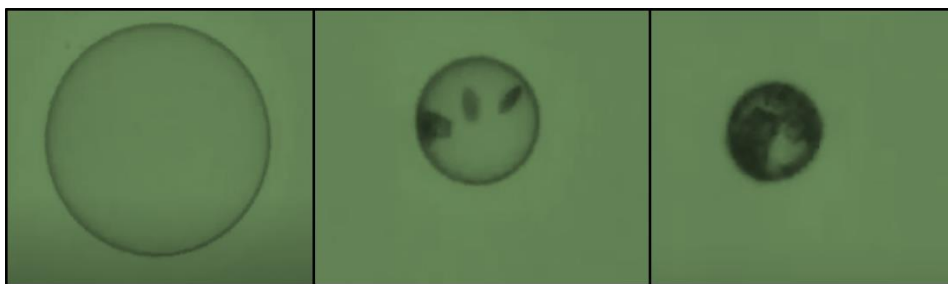
Figure 4.13: Shrinking behavior of the droplet formed by the precursor solution in the silicone oil.
