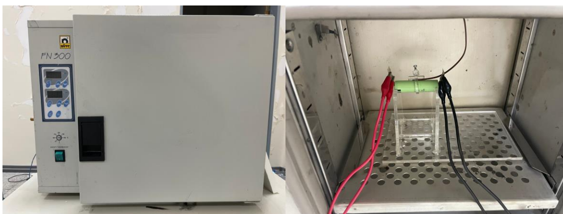
Figure 3.2. Battery connections and placement inside the oven.
